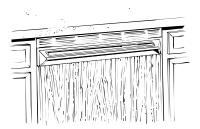
**4.** Slide refrigerator into recess after leveling it and plugging its power cord into electrical outlet.
